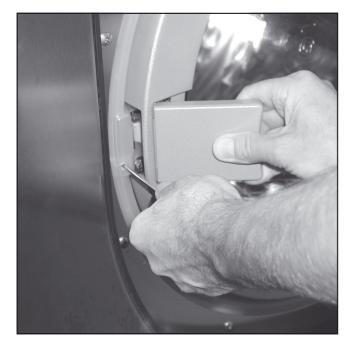
■ Insert a screwdriver (head approx. 4 mm) into the opening beside the door lock so that the head engages with the notch of the door release mechanism. Turning the screwdriver slightly anti-clockwise will unlock the door.
