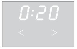
■ Touch the < or > sensor control repeatedly until the required programme running time appears in the time display.
