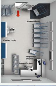
A typical room layout for a barrier wash system with clean and dirty sides
