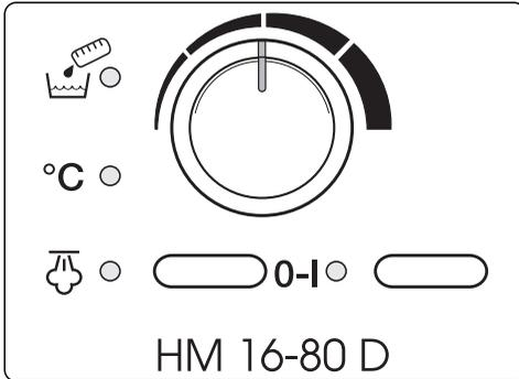
The **I-O** "On-Off" button is used for switching the ironer on and off.
