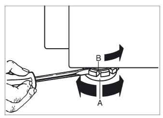
The screw feet A can be adjusted to align it.
